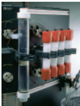
Fig. 51. Four HiPrep 26/10 Desalting columns connected in series.
